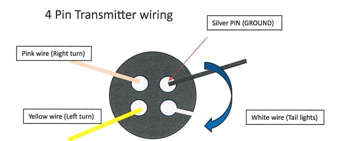
This is the back of the plug where you can see wires. Start with silver pin and go clockwise with these colors
